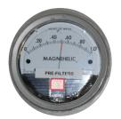
MEGApleat® M8 filters in service over eight months show a resistance of only 0.5" w.g. Standard capacity filters would have been changed out three times at this point.
